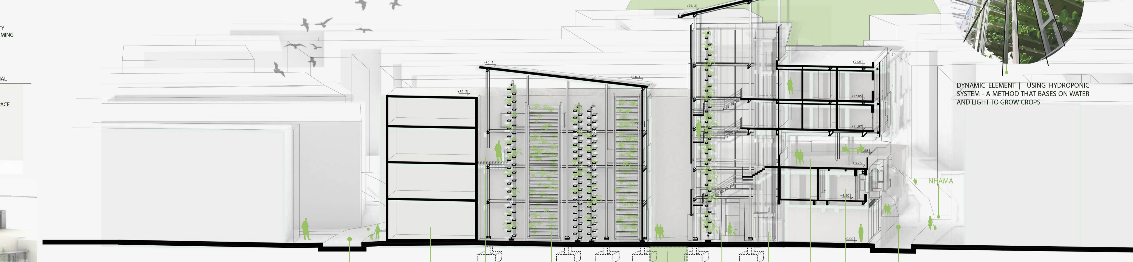
SECTION A-A SCALE 1:250 Passes through the existing structure and the addition of the residence and courtyard between the buildings - with the vertical greenhouse
